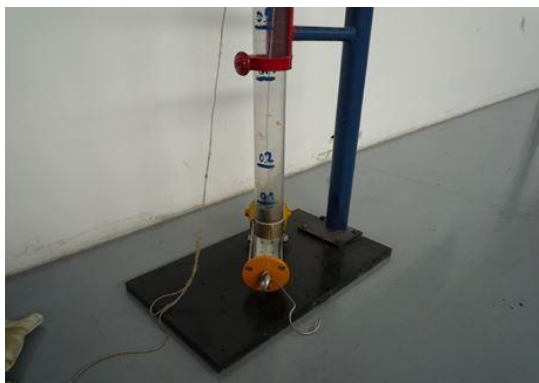
Fig.3. Lamp subjected to resistance to impact test
